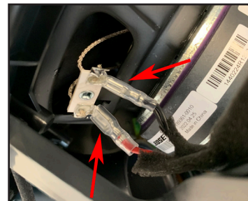
Figure 20. 2 Cable Harnesses Removal
