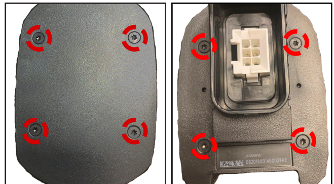
Figure 25. Both Ends of Endcaps Screws Removal
