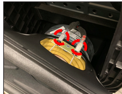
Figure 24. Press the White Fastener
