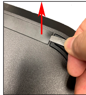
Figure 7. PC Sheets Removal
