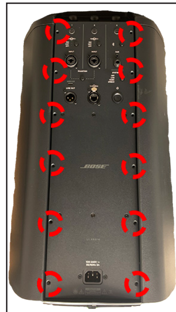
Figure 11. I/O Panel Assy Screws Removal
