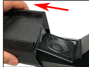
Figure 27. Array Grille Removal
