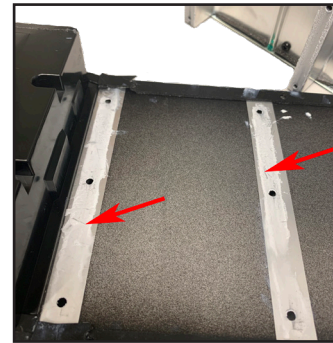
Figure 16. Heat Sink Thermal Grease
