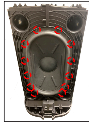
Figure 23. Woofer Screws Removal
