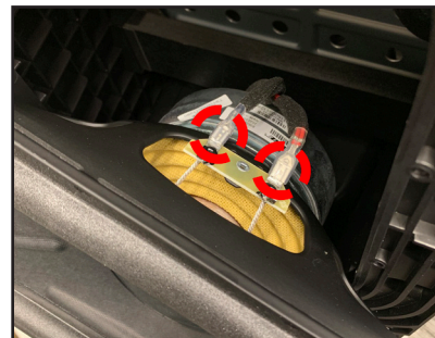
Figure 24. Press the White Fastener
