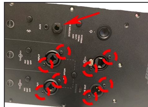
Figure 21. 4 Jacks and Jack Socket Nut Removal
