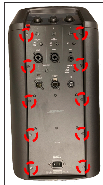
Figure 11. I/O Panel Assy Screws Removal
